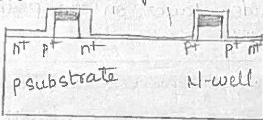
Form a metal doped layers for the drain & gate elements
