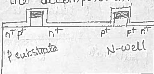
Removal of oxidation layer to form source, drain and gate elements
