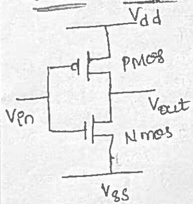
For the CMOS Inverter, we know the CMOS is a combination of both nMOS and pMOS transistors.
